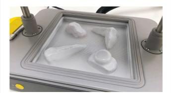
Carefully cut away the excess around the car designs with a pair of scissors.
