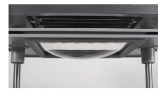
Allow the plastic to cool and remove the whole thing from the FormBox. Gently remove the models. Mayku FormBox
