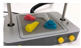
When the plastic is ready you will see ripples at the edges of the sheet and a droop in the middle. Form the models with the Mayku Form Sheet.
